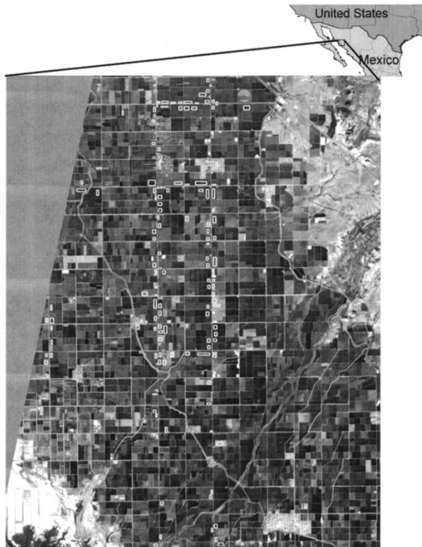
Fig. 1. ALI panchromatic image of the Yaqui Valley study region. Fields used to compare ALI and ETM+ radiance are delineated by white lines.
